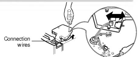
2) Remove keeper by rotating it clockwise (①) and then remove the upper hinge by lifting it up (②).
