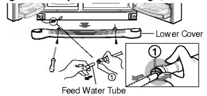
Remove the lower cover by lifting upward, and then pull up the feed water tube while pressing area ① shown in the figure to the right.
