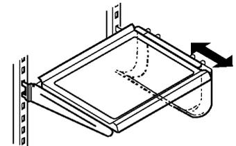
The Refrigerator compartment shelf is movable so that you can place it at a proper height according to the space you need for different food items..
