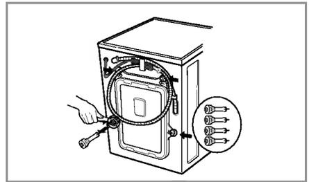
3. Take out the 4 bolts along with the rubber bungs by slightly twisting the bung. Keep the 4 bolts and the spanner for future use.
