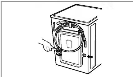
2. Unscrew the 4 bolts with the spanner supplied.
