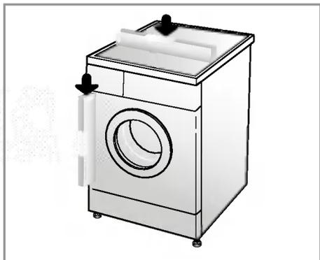
1. Adjusting the washing machine level properly prevents excessive noise and vibration.
