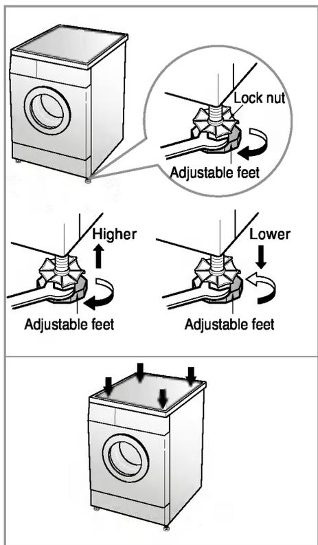
2. If the floor is uneven, adjust the adjustable feet as required. (do not insert pieces of wood etc. under the feet)
