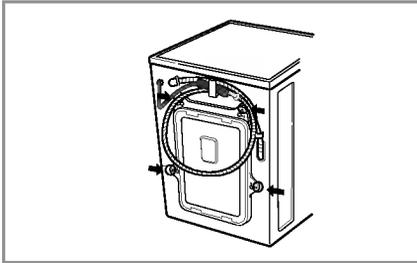
1. To prevent internal damage during transport, the special 4 bolts are locked. Before operating the washer, remove the bolts along with the rubber bungs.
