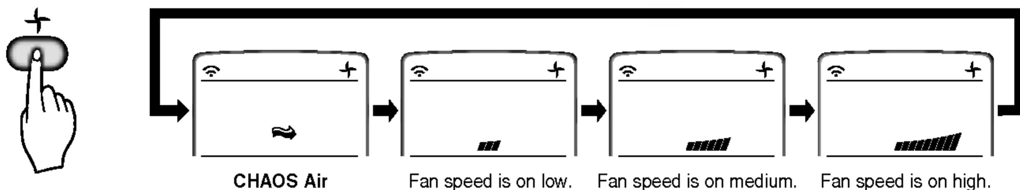
**NOTICE** CHAOS Air economizes power consumption and prevents overcooling. The fan speed is automatically changed from high to low or vice versa, depending on the ambient temperature.
