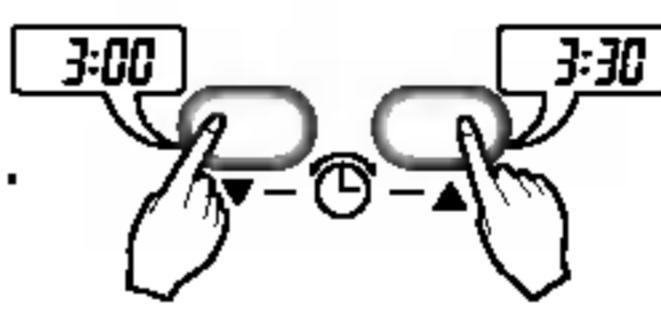
5. To set the selected time, press the Timer setting button aiming the remote controller at the signal receptor.
