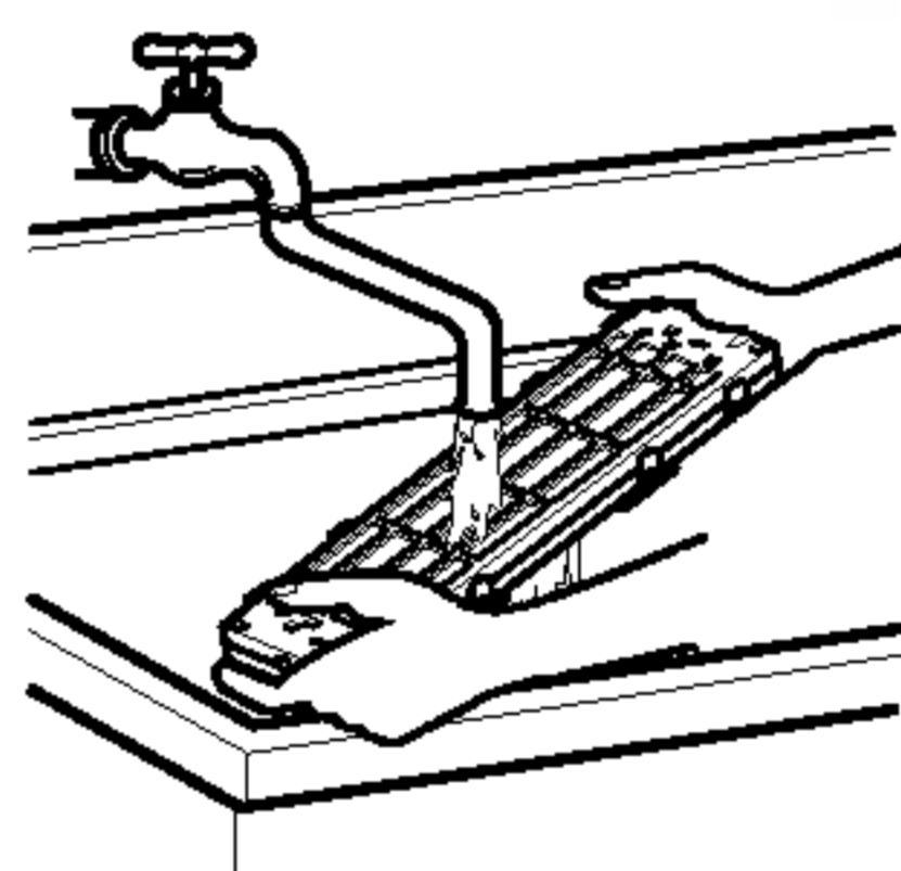
4. Insert the Plasma Filter after perfectly drying it in shade. Now insert Air Filter and close the front panel completely by matching the hook.
