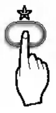
2. The Timer is programmed in one-hour increments by pressing the Sleep Mode Auto button 1 to 7 times. The sleep mode is available for 1 to 7 times. To alter the time period in steps of 1 hour, press the Sleep Mode Button while aiming at air conditioner.
