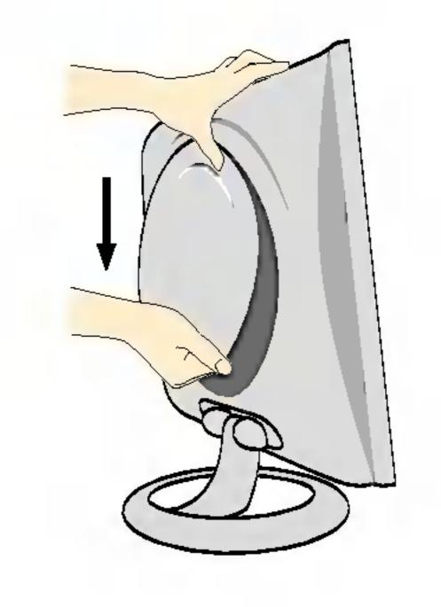
1. Separate the back cap by sliding its lower section downward as shown in the picture.
