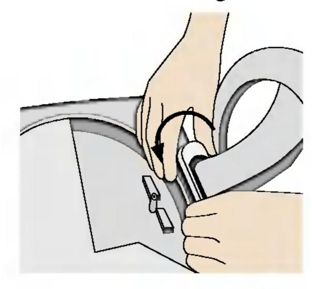
2. Slide off the lower section of the cover base with two hands as shown in the picture.
