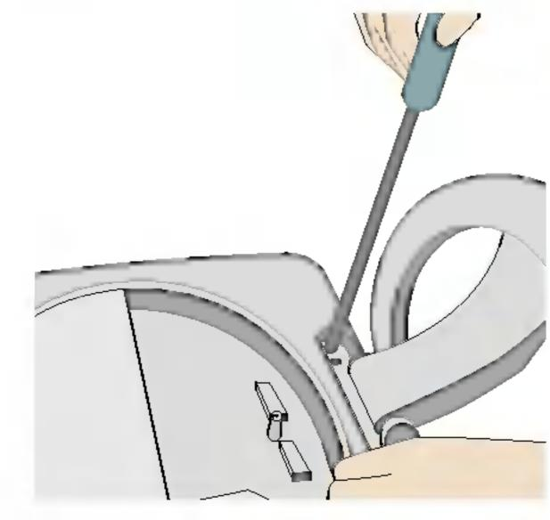
3. Separate the stand base using a screwdriver as shown in the picture.
