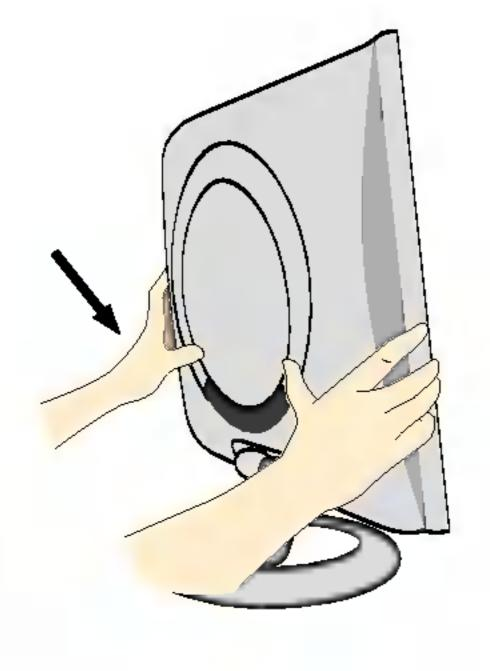
4. Insert the back cap along the bottom grooves on both sides, holding the bottom.
