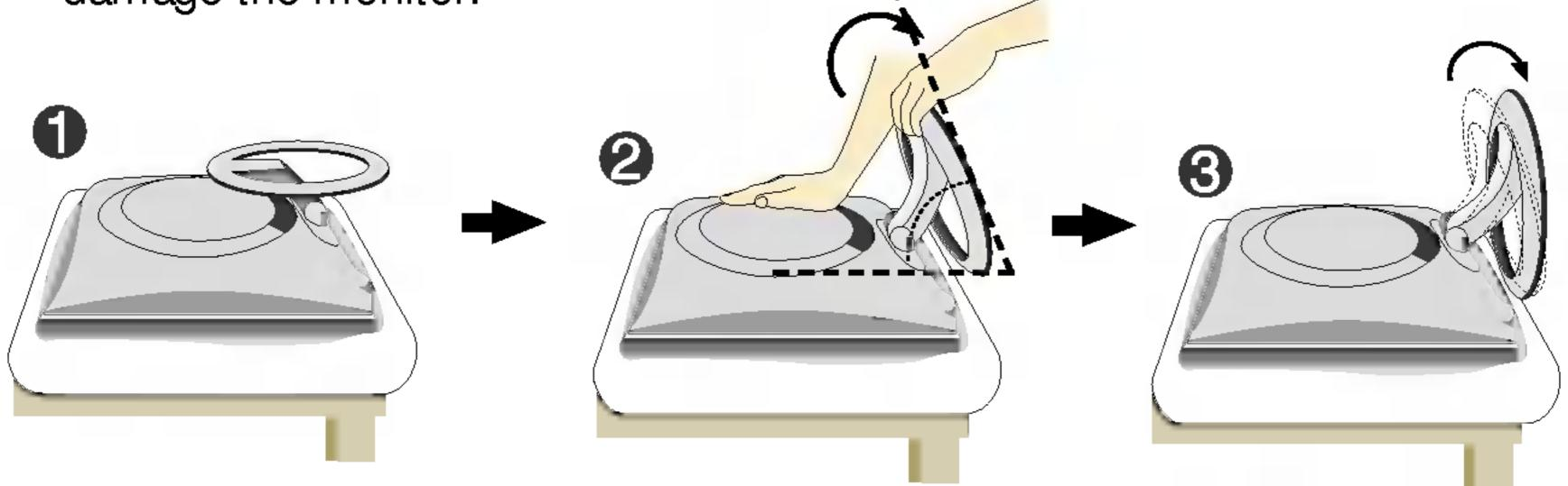
4. Place the monitor upright and adjust the stand base angle as desired. Adjust the stand base angle holding the monitor head part with both hands.
