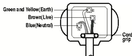
As the colours of the wires in the mains lead of this apparatus may not correspond with the coloured markings identifying the terminals in your plug, proceed as follows:
