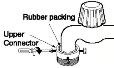
3. Push the water supply hose vertically upwards so that the rubber packing within in the hose can adhere completely to the tap and then tighten it by screwing it to the right.
