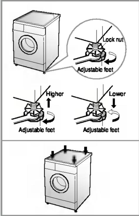
1. Adjusting the washing machine level properly prevents excessive noise and vibration.
