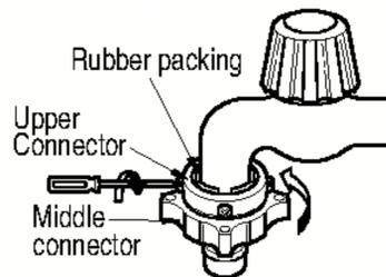
3. Connect the water supply hose to the middle connector, pushing the plate down.
