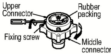
2. Push the upper connector up till the rubber packing is in tight contact with the tap. Then tighten the 4 screws.
