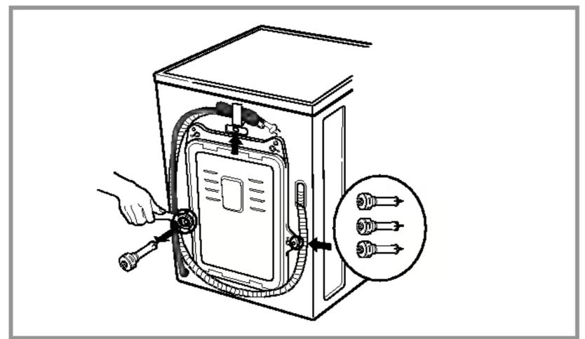
3. Take out the 3 bolts along with the rubber bungs by slightly twisting the bung. Keep the 3 bolts and the spanner for future use.
