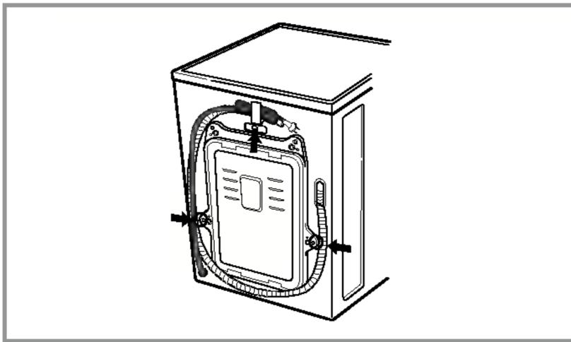
1. To prevent internal damage during transport, the special 3 bolts are locked. Before operating the washer, remove the bolts along with the rubber bungs.
