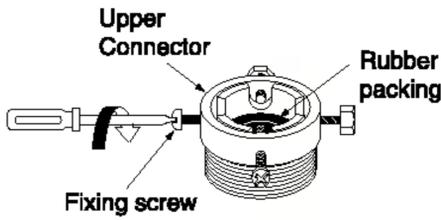
2. Push the connector up till the rubber packing is in tight contact with the tap. Then tighten the 4 screws.
