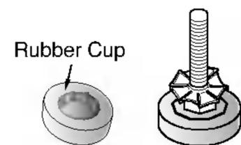
\* *Insert the rubber cups to reduce vibration.*
