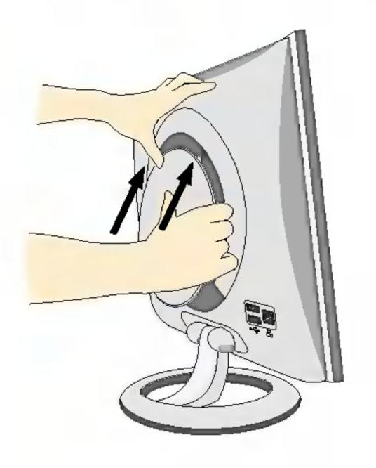
**3.** After the cables are connected, set the back cap into the groove of the upper section and reassemble by pushing upward.
