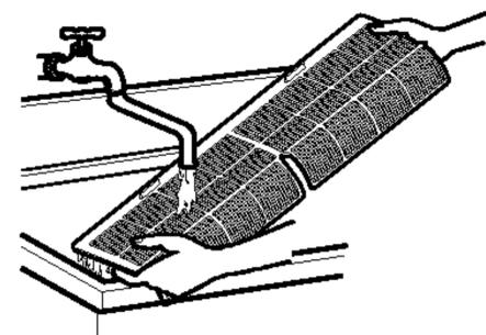
5. Reinstall the air filter dried at the shade and then close the panel.
