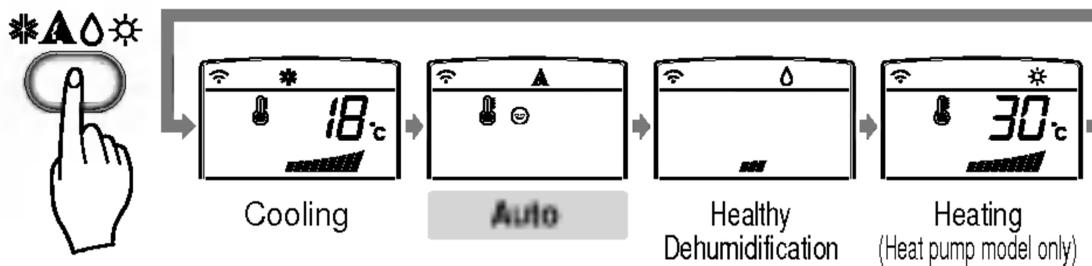
**3** The temperature and fan speed are automatically set by the electronic controls based on the actual room temperature. If you want to change the set temperature, press the Room Temperature Setting buttons. The cooler or warmer you feel, the more times (up to two times) you should press the button. The set temperature will be changed automatically.
