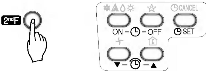
**3** 2nd function disappears in a short time automatically or when the button is pressed again.
