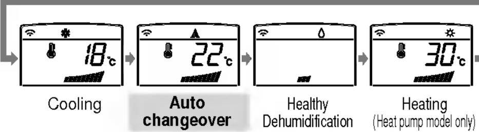
**3** Close the door of the remote controller. Set the temperature lower than the room temperature. The temperature can be set within a range of 18°C~30°C at intervals of 1°C.
