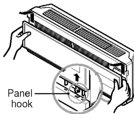
3. Remove air filter and then pull out the nano plasma filter.
