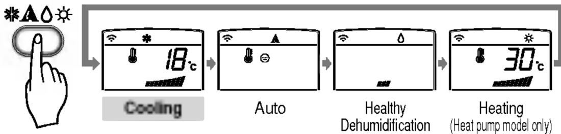
**3** Close the door of the remote controller. Set the temperature lower than the room temperature. The temperature can be set within a range of 18°C~30°C at intervals of 1°C.
