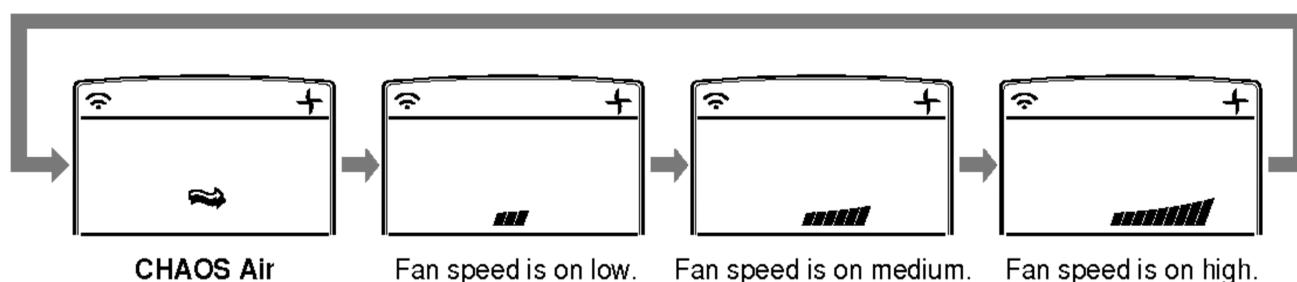
**NOTICE** CHAOS Air economizes power consumption and prevents overcooling. The fan speed is automatically changed from high to low or vice versa, depending on the ambient temperature.
