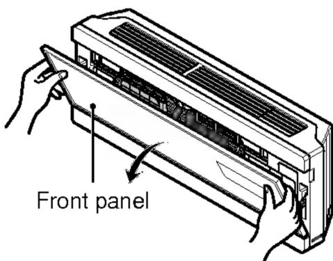
2. Put up the front panel. The hook of panel comes off.
