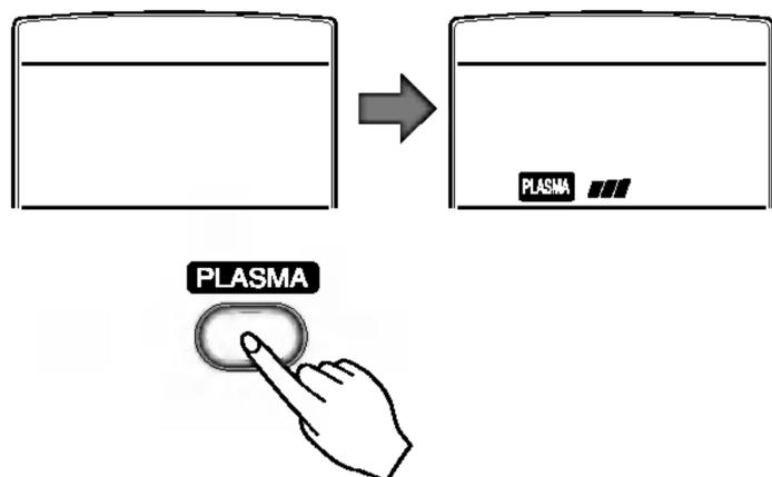
If you press the only NANO PLASMA button, only NANO PLASMA purification function operates.
