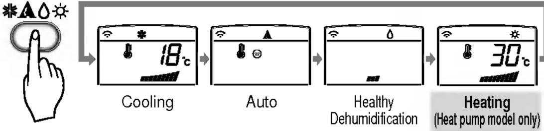
**3** Close the door of the remote controller. Set the temperature higher than the room temperature. The temperature can be set within a range of 16°C~30°C at intervals of 1°C.
