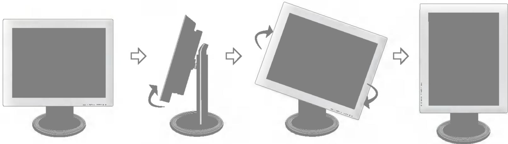
\* Make sure not to touch the floor when the head rotates to use the Pivot function.
