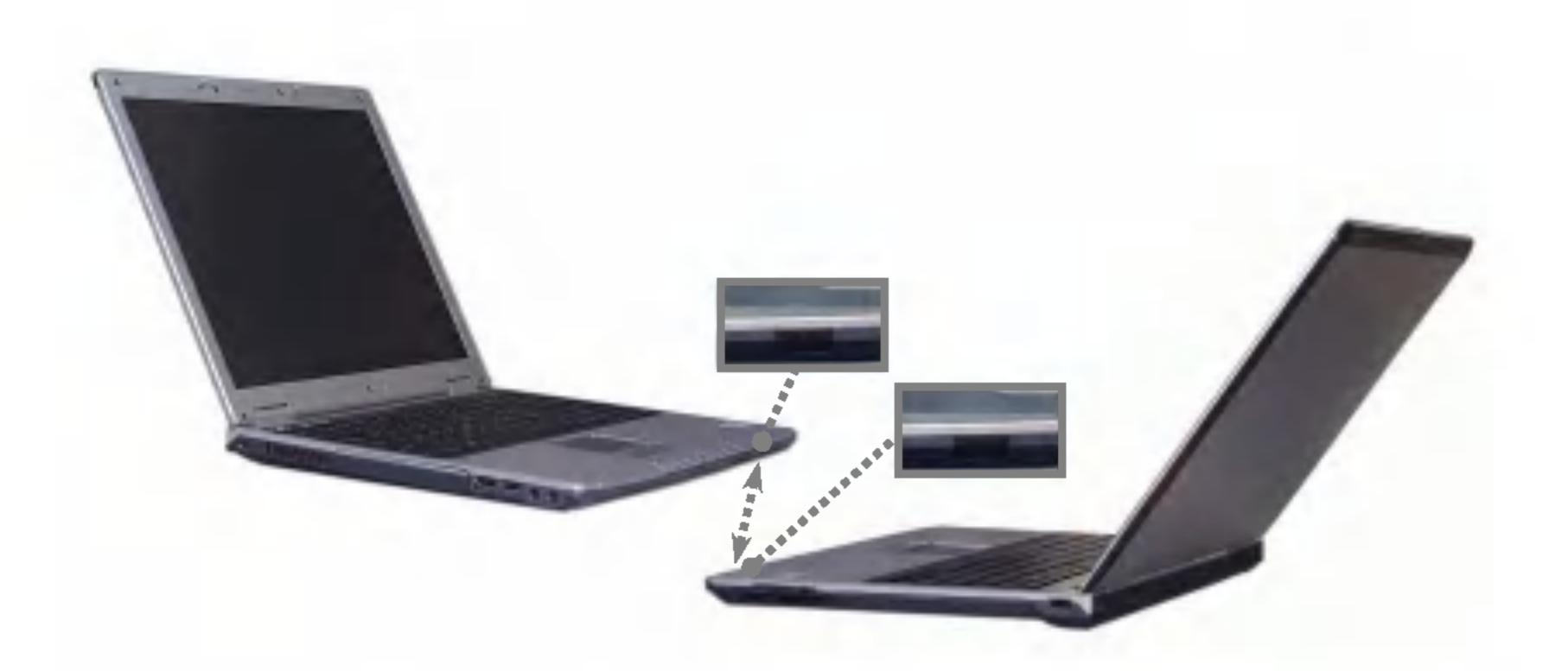
The distance and the beam angle between the ports must be less than 1m and smaller than +-15 degrees respectively.
