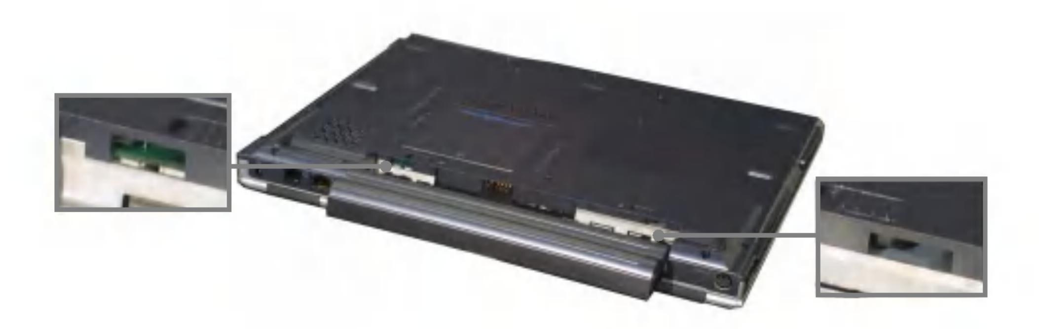
3. Gently push the battery pack into the slot until it clicks. The battery pack is inserted. You can lock the battery pack in place by pushing the left battery latch in the direction shown above. If you hear a click, the battery pack is locked in.
