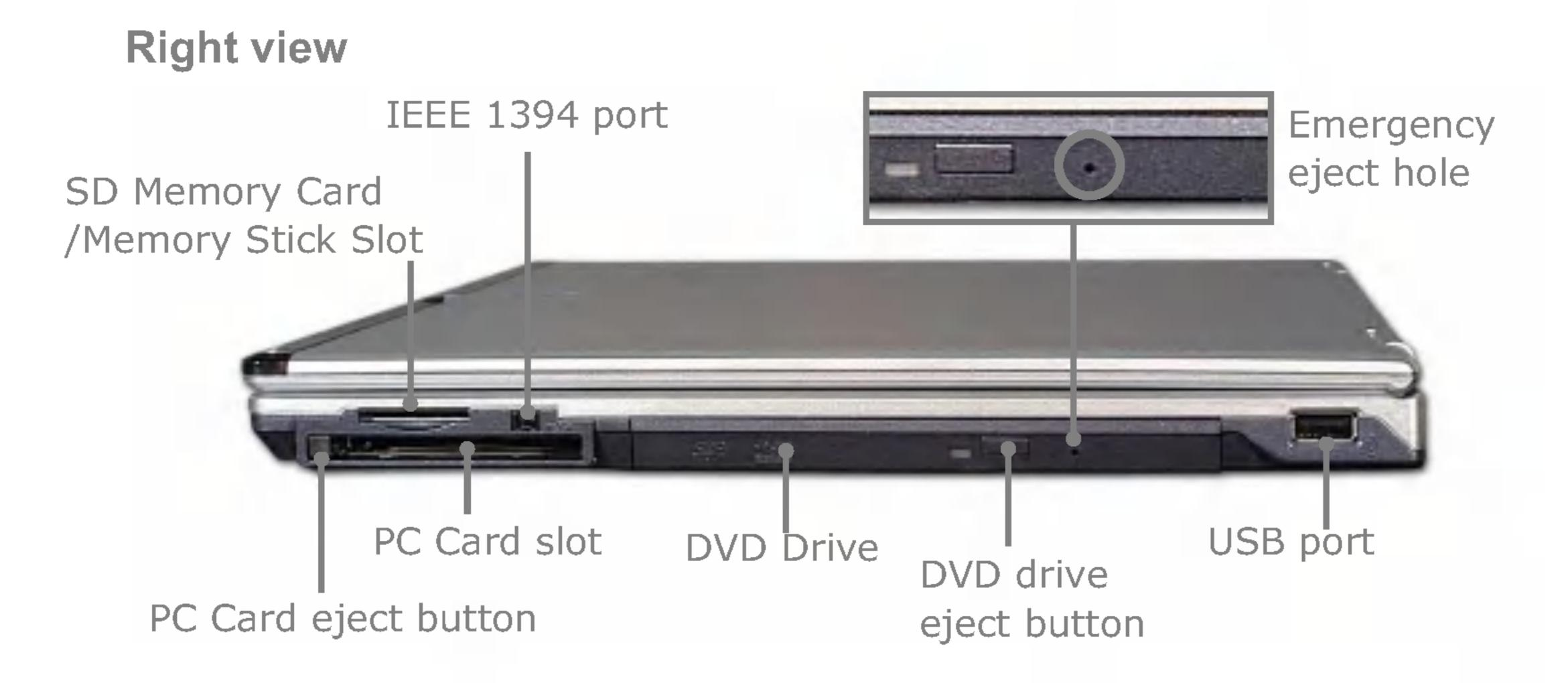
Emergency eject hole: Insert a thin and hard pin into this hole, and you can open the disc tray manually.
