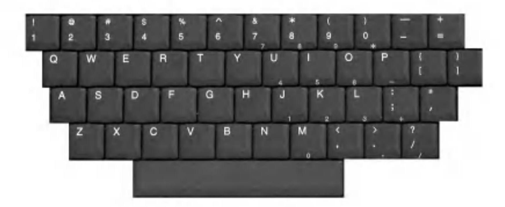
Embedded numeric keys: You can press the combination of Fn and ScrLk keys to enable the embedded numeric keypad. Num Lock indicator lights up and enables you to use the embedded numeric keypad shown below. You can press the combination of Fn and ScrLk keys again to disable the embedded numeric keys. (To use the numeric keys, you must set the Advanced -> Internal Keypad setting to Enabled in the BIOS Setup Utility.)
