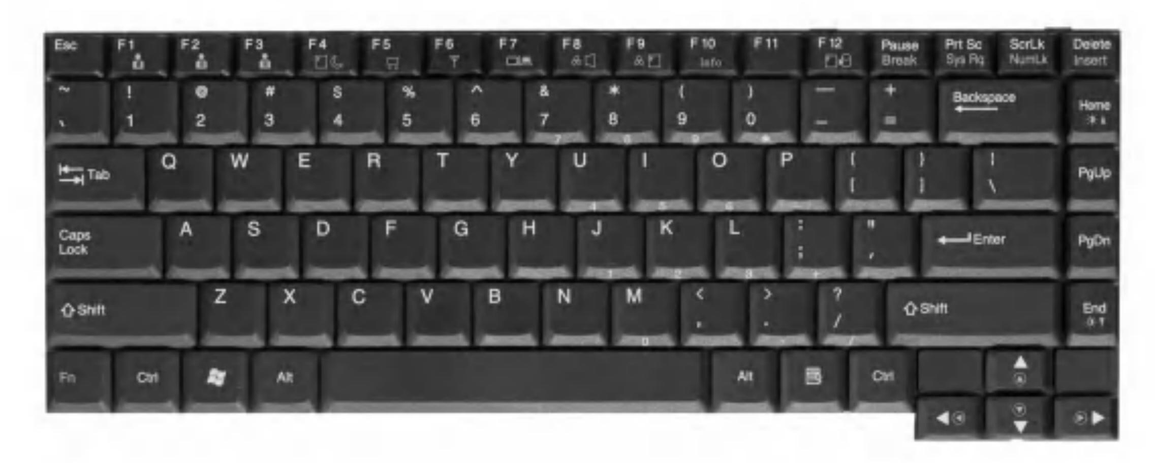
Function keys: Function keys enable you to perform different operations depending on the operating system and application program you use.
