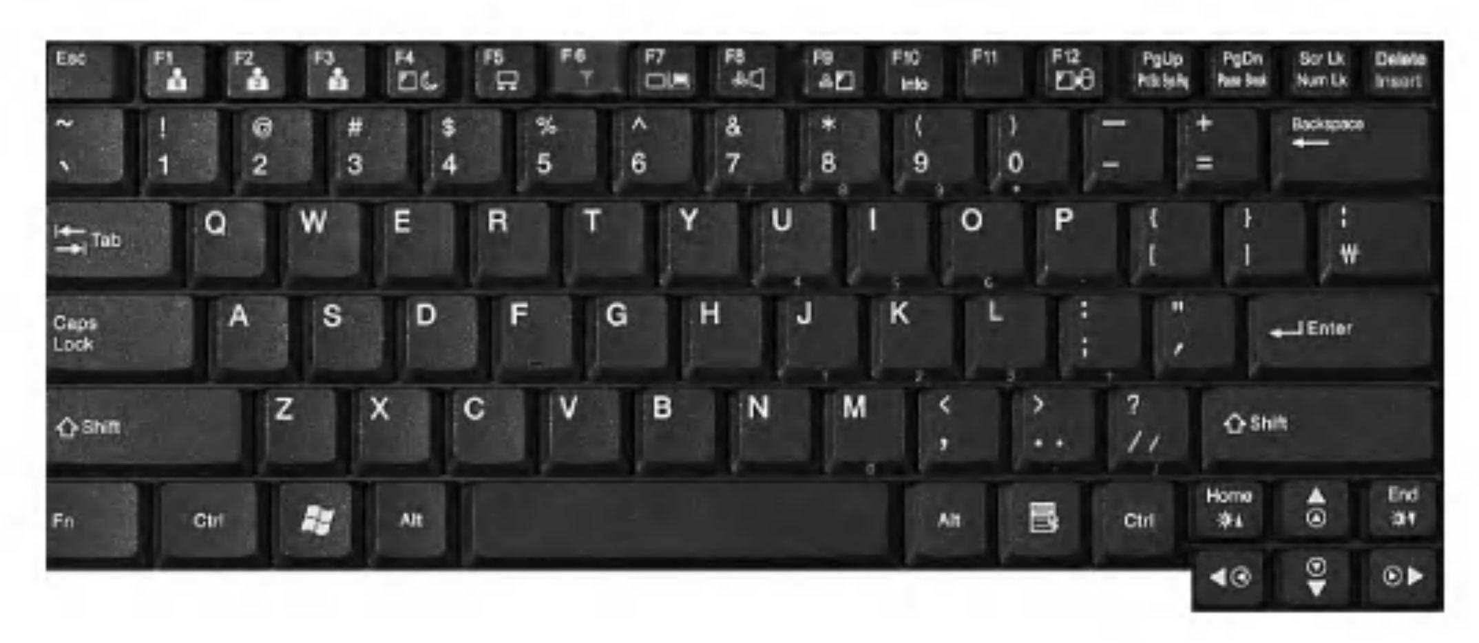
Function keys: Function keys enable you to perform different operations depending on the operating system and application program you use.
