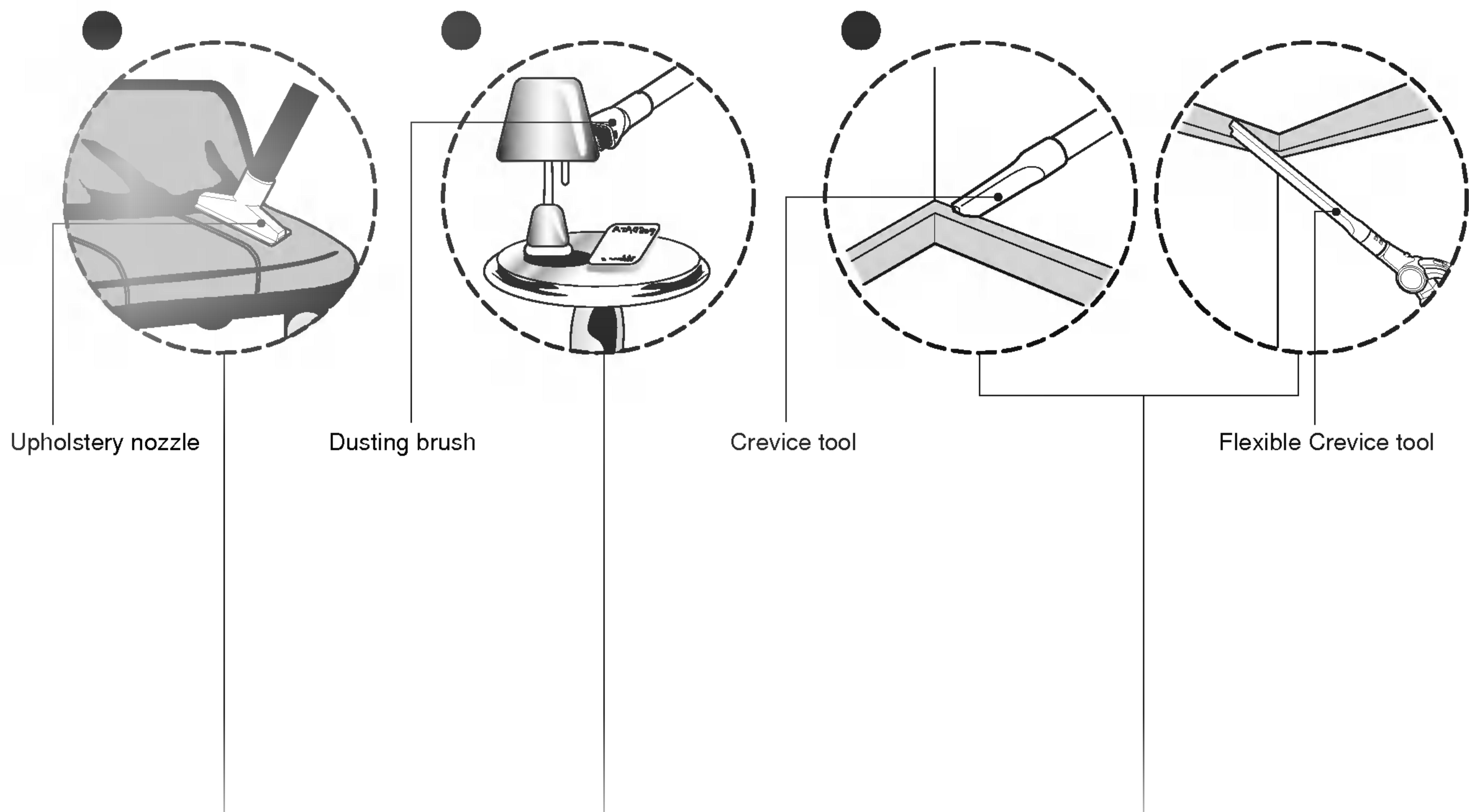
Upholstery Nozzle is for vacuuming upholstery, mattresses, etc. The thread collectors help to pick up the threads and fluff.
