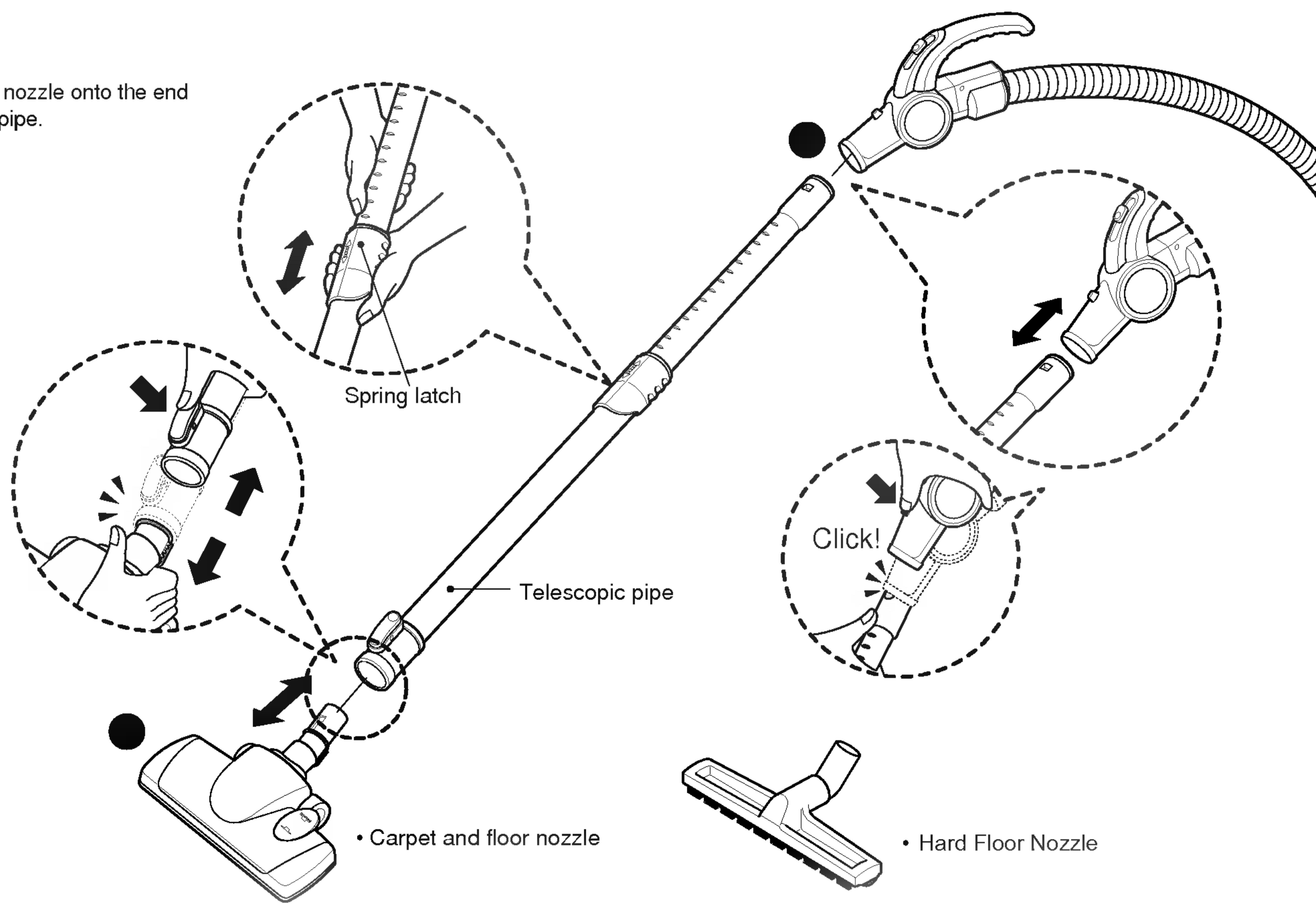
Push the nozzle onto the telescopic pipe.
