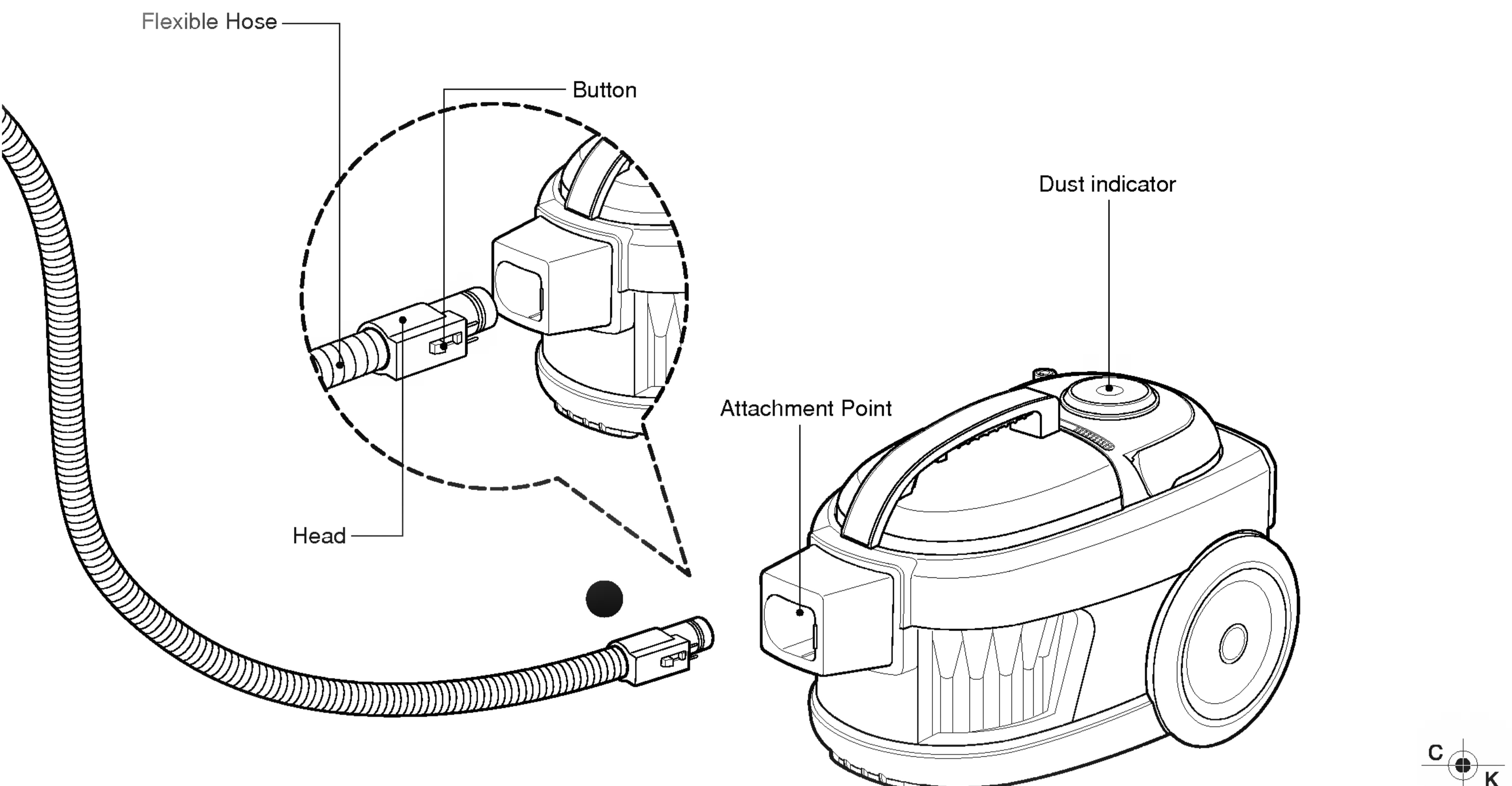
Push the end of the head on the flexible hose into the attachment point on the vacuum cleaner. To remove the flexible hose from the vacuum cleaner, press on the button situated on the head, then pull the head out of the vacuum cleaner.
