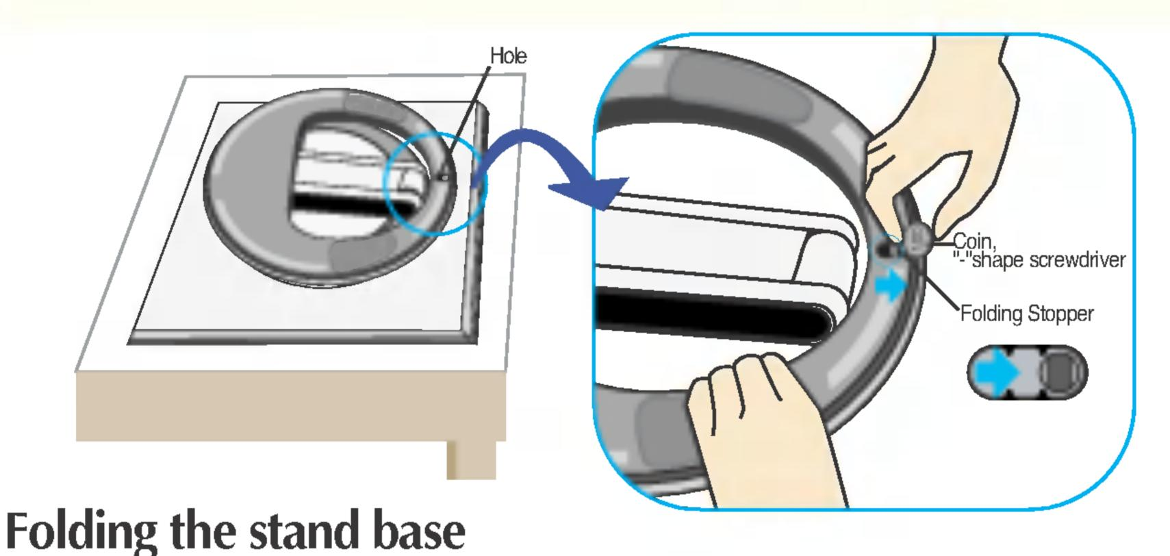
1. To fix a stand, push the folding stopper inwards until you hear the 'click' sound using a coin of '-shape screw driver, while pressing down the stand base to the monitor.
