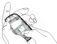
To remove the SIM card
