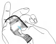
To insert the SIM card
