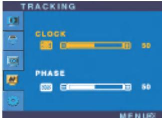
A screenshot of the OSD tracking adjustment menu. It shows two horizontal sliders: 'CLOCK' and 'PHASE', both set to 50. The background shows a blue grid pattern. The menu bar at the bottom says 'MENU'. | <b>CLOCK</b> To minimize any vertical bars or stripes visible on the screen background. The horizontal screen size will also change.<br><b>PHASE</b> To adjust the focus of the display. This item allows you to remove any horizontal noise and clear or sharpen the image of characters. |
