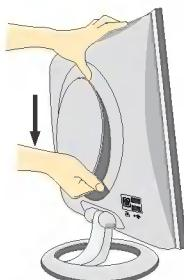
1. Separate the back cap by sliding its lower section downward as shown in the picture.
