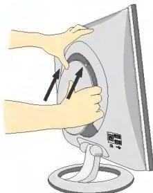
3. After the cables are connected, set the back cap into the groove of the upper section and reassemble by pushing upward.
