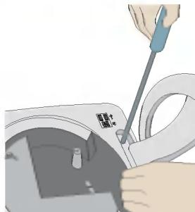
3. Separate the stand base using a screwdriver as shown in the picture.
