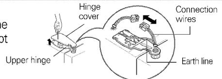
2) Remove the keeper by rotating it counter clockwise (①) and then lifting the upper hinge up (②).
