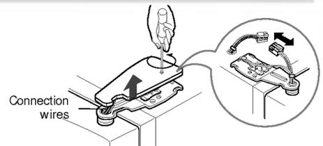
2) Remove keeper by rotating it clockwise (①) and then remove the upper hinge by lifting it up (②).
