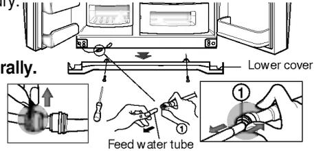
**Remove lower cover and then feed water tube**
