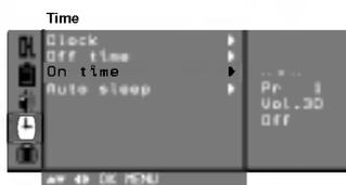
4. Press the **▶** button and then **▲ / ▼** button to adjust the minute.
