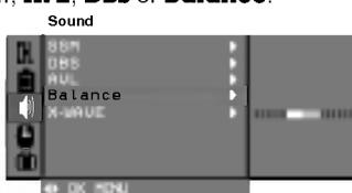
3. Make desired adjustment with the **◀ / ▶**, **▲ / ▼** or **OK** button on each pull-down menu.
