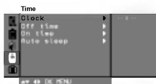
3. Press the **▶** button and then **▲ / ▼** button to adjust the hour.
