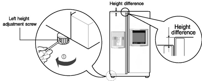
**If the freezer compartment door is higher than the refrigerator compartment door**
