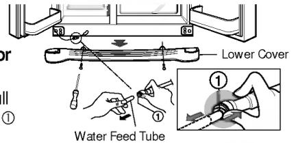
**Remove lower cover and water feed tube**
