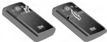
To insert the USIM card To remove the USIM card
