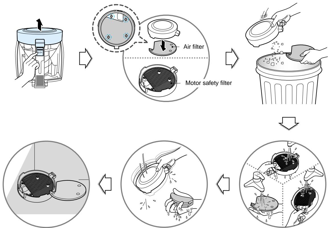
If the indicator is lighted on after cleaning the dust tank , clean the air filter and motor safety filter. The air filter and motor safety filter are located at the bottom of dust tank cap in above figure.
