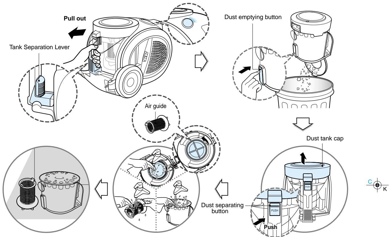
Check the indicator is lighted on after emptying the dust tank. If the indicator is lighted on when dust tank is not filled, firstly clean the dust tank and air guide as follows.
