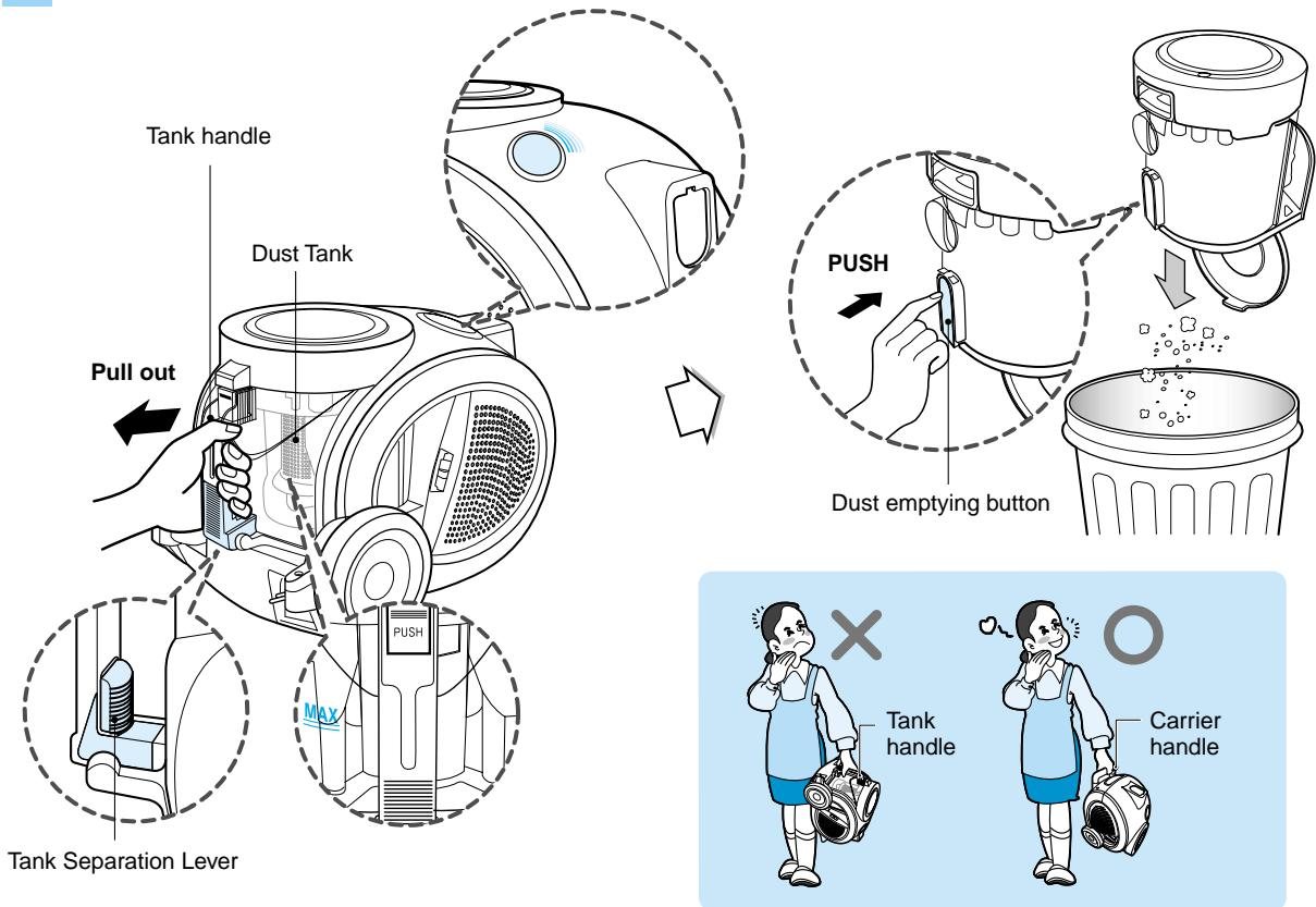
The dust tank needs emptying when dust reaches the "MAX" position on the dust tank or indicator is lighted on.
