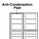
• Especially after installation or when ambient temperature is high, the fridge-freezer may feel hot, which is guite normal.
