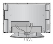
Reinstall the CABLE MANAGEMENT as shown.
