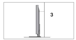
Use a sturdy rope (not provided as parts of the product, must purchase separately) to tie the product. It is safer to tie the rope so it becomes horizontal between the wall and the product.
