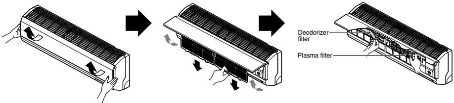
**Type 2:** Pull the front panel from both sides as shown.
