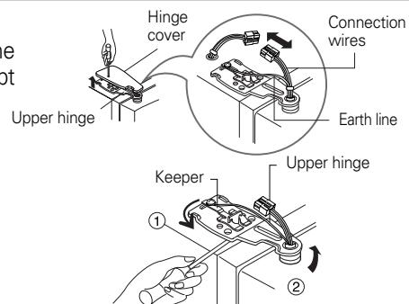
2) Remove the keeper by rotating it counter clockwise (①) and then lifting the upper hinge up (②).
