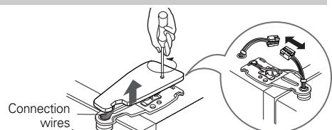
2) Remove keeper by rotating it clockwise (①) and then remove the upper hinge by lifting it up (②).
