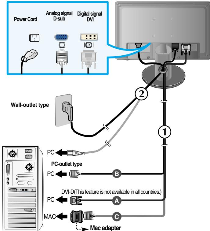
For Apple Macintosh use, a separate plug adapter is needed to change the 15 pin high density (3 row) D-sub VGA connector on the supplied cable to a 15 pin 2 row connector.
