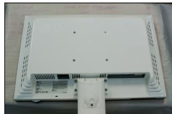
2. Separate the stand using a screwdriver as shown in the picture.
