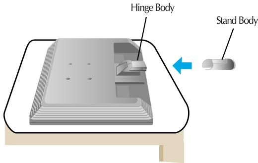
3. Assemble the Stand Base(Front, Rear) into the Stand Body in the correct direction. However, the body of the stand will be fixed firmly only when it is connected to the base.
