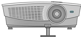
1. While pressing the foot adjusting button, raise or lower the projector to place the screen image in the proper position.
