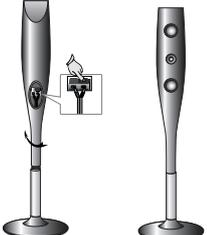
3. Fix the speaker to the stand by rotating the speaker. Connect the speaker cord to the appropriate terminals on the speaker.
