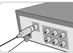
Connect one of the DVD unit's **DIGITAL OUT** jacks to the corresponding in jack on your amplifier. Use an optional digital audio cable.
