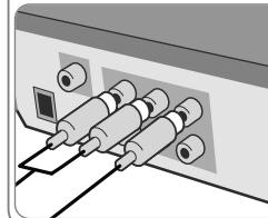
Connect to the external device had **AUDIO IN** jacks. The unit's **AUDIO OUT(R/L)** jacks are colour coded (red for right audio and white for left audio). Connect the **VIDEO OUT** jack on the unit to the corresponding input jack on your TV using a Video cable.
