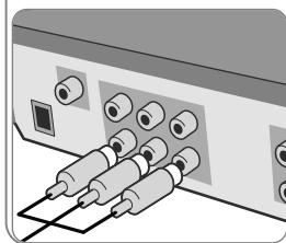
Connect the **COMPONENT/PROGRESSIVE SCAN OUTPUT** jacks on the unit to the corresponding input jacks on your TV using a Y PB PR cable.
