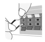
3 Connect the wires to the speakers.
