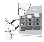
2 Connect the wires to the speakers.
