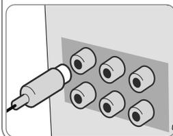
Connect the VIDEO OUT-PUT jack on the active woofer to the corresponding input jack on your TV using a Video cable.
