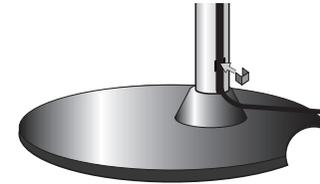
Fix the unit tighten 3 screws (3 x 14) on the rear side of the stand.
