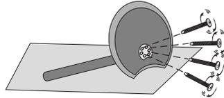
Insert the cable holder in the hole on the stand.
