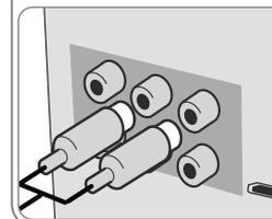
The unit's Audio jacks are colour coded (red for right audio and white for left audio). If your TV has only one input for audio (mono), connect it to the left (white) audio jack on the unit.
