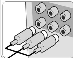
Connect the COMPONENT VIDEO OUT jacks on the active woofer to the corresponding input jacks on your TV using a Y PB PR cable.
