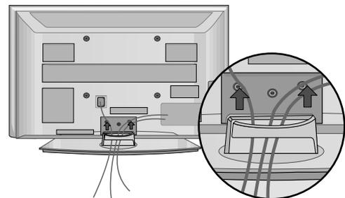
\* For the 42PG1\*\*\* model, press the center of the CABLE MANAGEMENT CLIP and then lift up it.
