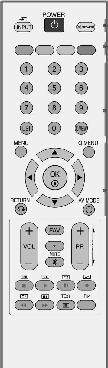
**POWER** Switches the TV on from standby or off to standby.
