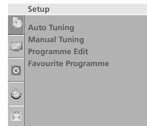
2 Press the  $\triangleright$  button and then  $\wedge/\vee$  button to select **Manual Tuning**.
