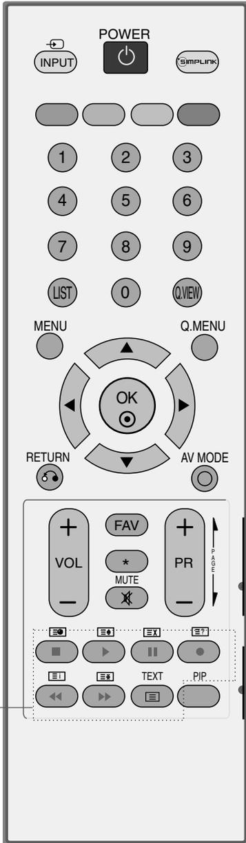
**1 TELETEXT BUTTONS** These buttons are used for teletext. For further details, see the 'Teletext' section.
