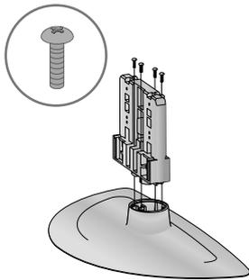
**4** Fix the 4 bolts securely using the holes in the back of the TV.
