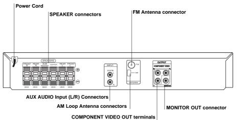
Connect to a TV with Y PB PR inputs.
