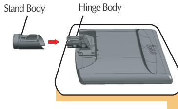
3. Assemble the Stand Base (Front, Rear) into the Stand Body in the correct direction, then tighten the screw as shown in the picture.
