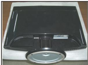
3. Slide the Cable Deco Cover out from the stand body.
