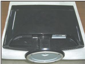
4. Loosen the screw, then take off the stand base from stand body.
