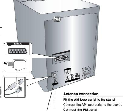
The reception will be at its best when the two loose ends of the aerial are in a straight line
