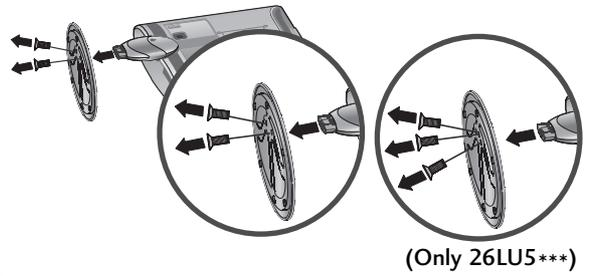
**3** Loosen the bolts and then detach the Cover Base from TV.
