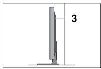
Use a sturdy rope to tie the TV. It is safer to tie the rope so it becomes horizontal between the wall and the TV.
