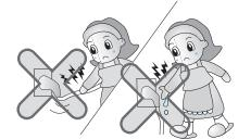
Remove water or dust from the power plug and insert it with the ends of the pins securely connected.
