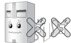
Do not allow the power cord bent or pressed by the heavy object to be damaged.
