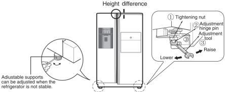
Do not adjust the height excessively. You can lose the hinge pin. (Height adjustable range: Maximum of 5mm)
