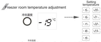
Whenever pressing O button, setting is repeated in the order of  $(-19^{\circ}\text{C} \rightarrow -20^{\circ}\text{C} \cdots \rightarrow -23^{\circ}\text{C} \rightarrow -15^{\circ}\text{C} \cdots \rightarrow -19^{\circ}\text{C}).$
