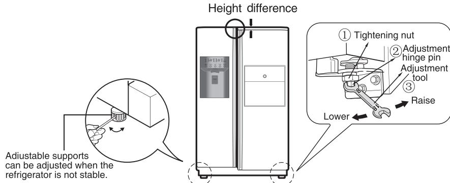
**Do not adjust the height excessively. You can lose the hinge pin.
