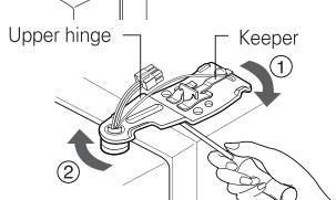
3) Remove the refrigerator compartment door by lifting it up.
