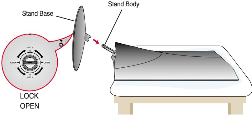
3. Once assembled take the monitor up carefully and face the front side
