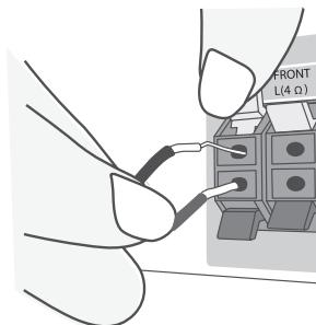
Connect the red end of each wire to the terminals marked +(plus) and the black end to the terminals marked -(minus).
