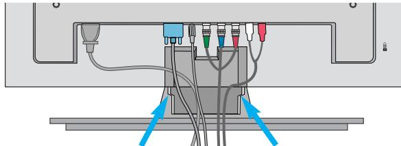
2. Fit the cable guide to the back to help manage the cables.
