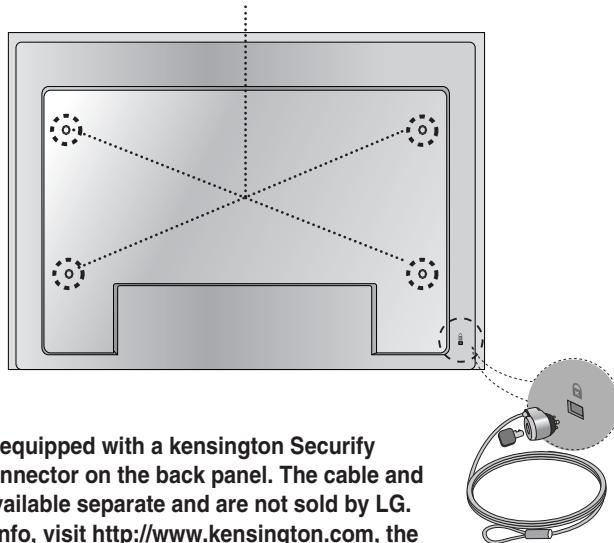
The Set is equipped with a kensington Security System connector on the back panel. The cable and lock are available separate and are not sold by LG. For more info, visit <http://www.kensington.com>, the internet home page of the Kensington company.
