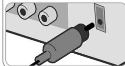
Connect the unit's OPTICAL IN jack to the optical out to jack on your TV (or Digital Device etc.)
