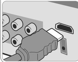
Connect the HDMI OUTPUT jack on the unit to the HDMI input jack on a HDMI compatible TV using a HDMI cable.
