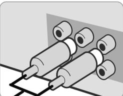
The unit's Audio jacks are colour coded (red for right audio and white for left audio). If your TV has only one input for audio (mono), connect it to the left (white) audio jack on the unit.
