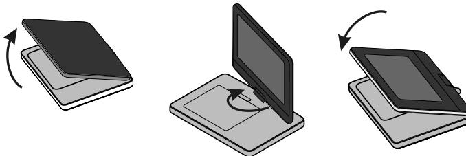
To revolve the LCD panel, place the unit on a stable and even surface such as on a table. Push the LCD panel up and then lift it into a vertical position. Revolve the LCD panel clockwise slowly 180 degrees. If you need, fold the LCD panel after revolving it.
