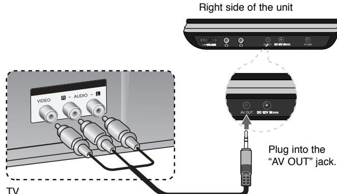
**Note:** The signal does not come out from AV OUT jack when the unit is set to [TV] mode.
