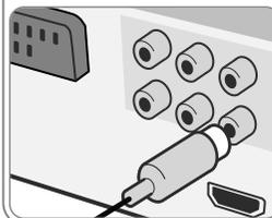
Connect the VIDEO OUTPUT (MONITOR) jack on the unit to the corresponding input jack on your TV using a Video cable.
