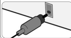
Connect the unit's OPTICAL IN jack to the optical out to jack on your TV (or Digital Device etc.)
