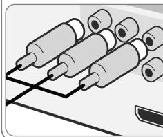
Connect the COMPONENT VIDEO (PROGRESSIVE SCAN) OUTPUT jacks on the unit to the corresponding input jacks on your TV using a Y PB PR cable.
