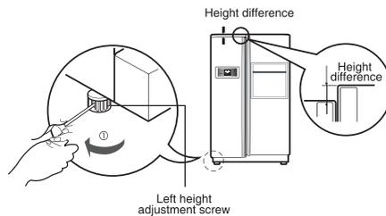
**If the freezer compartment door is higher than the refrigerator compartment door**
