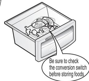
The meat compartment maintains the temperature at a lower point than the refrigerator compartment so that meat or fish can be stored fresh longer.
