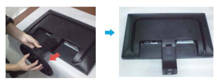
5. Pushing the PUSH button, Take the stand body from hinge body.
