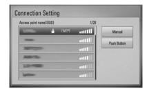
If you have security on your access point or wireless router, verify that the WEP or WPA key that was entered into the player matches the router's information exactly. You need to input the security code as necessary.
