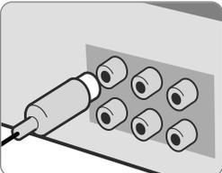
Connect the VIDEO OUTPUT(MONITOR) jack on the unit to the corresponding input jack on your TV using a Video cable.
