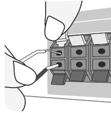
Connect the black end of each wire to the terminals marked -(minus) and the other end to the terminals marked +(plus).
