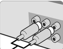
The unit's Audio jacks are colour coded (red for right audio and white for left audio). If your TV has only one output for audio (mono), connect it to the left (white) audio jack on the unit.
