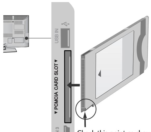
Check this point as shown and insert the CI Module.
