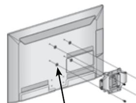
Place the ring spacers on the set before installing the wall mounting bracket so that the inclination of the backside of the set can be adjusted perpendicularly.
